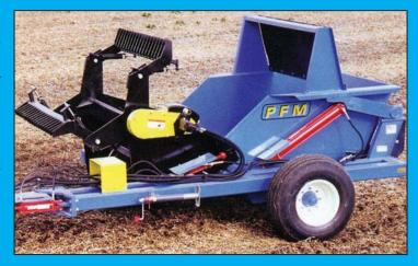
spring cushion action, individual hard surfaced teeth with heavy wall tube and carbon shafting and pins. The heavy duty pivot bucket hinges provide high strength and hopper stability. These features make the PFM rock picker the strongest and most durable on the market. It is built to stand up to the extra abuse demanded of rock removal equipment.
