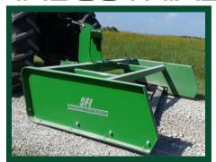
THE **SUPERIOR** INDUSTRIAL SCRAPERS ARE DESIGNED SIMILAR TO THE COMPACT GRADING SCRAPER, BUT IN A BIGGER HEAVIER FRAME. IT ALSO IS DESIGNED TO LOOSEN AND SMOOTH SURFACES. IT WILL TAKE DOWN HIGH SPOTS AND FILL IN LOW SPOTS WHILE MOVING DIRT FROM RIGHT TO LEFT WHICH MAKES IT REALLY HANDY ON GRAVEL DRIVEWAYS AND EVEN COUNTY ROADS.
