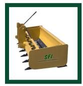
THE **SUPERIOR** 2C2 SERIES SCRAPERS ARE IDEAL FOR LANDSCAPE, TERRACE, BACK-FILL, SCARIFY, LEVEL OR GENERAL CLEAN -UP. AVAILABLE IN WIDTHS OF 60", 66", 72" & 76" FOR TRACTORS FROM 30 TO 60HP, 2 OR 4WD. AVAILABLE IN HYDRAULIC, MECHANICAL AND MANUAL VERSIONS.
