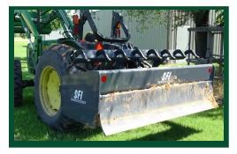
THE **SUPERIOR** 4C5 INDUSTRIAL BOX SCRAPER HAS A UNIQUE DESIGN THAT COMBINES THE RUGGEDNESS AND STRENGTH OF THE 4C4 HEAVY FIXED BACK PLATE WITH THE CONTROL OF THE 4C2 WITH FLOATING TAILBOARD.
